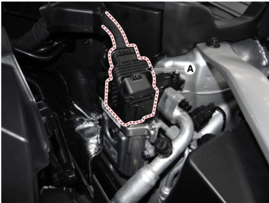
3. Remove the TCM (A) after loosening the nuts.
